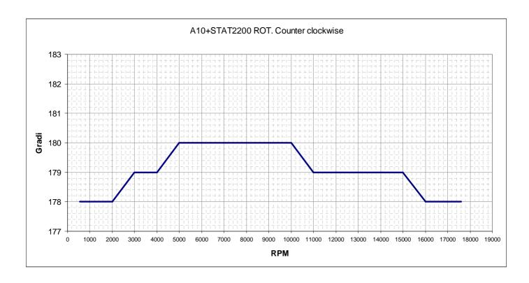
Figure shows the timing layout with speed of 5000rpm in counter clockwise rotation.
