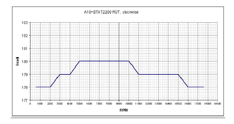
Figure shows the timing layout with speed of 5000rpm in clockwise rotation.
